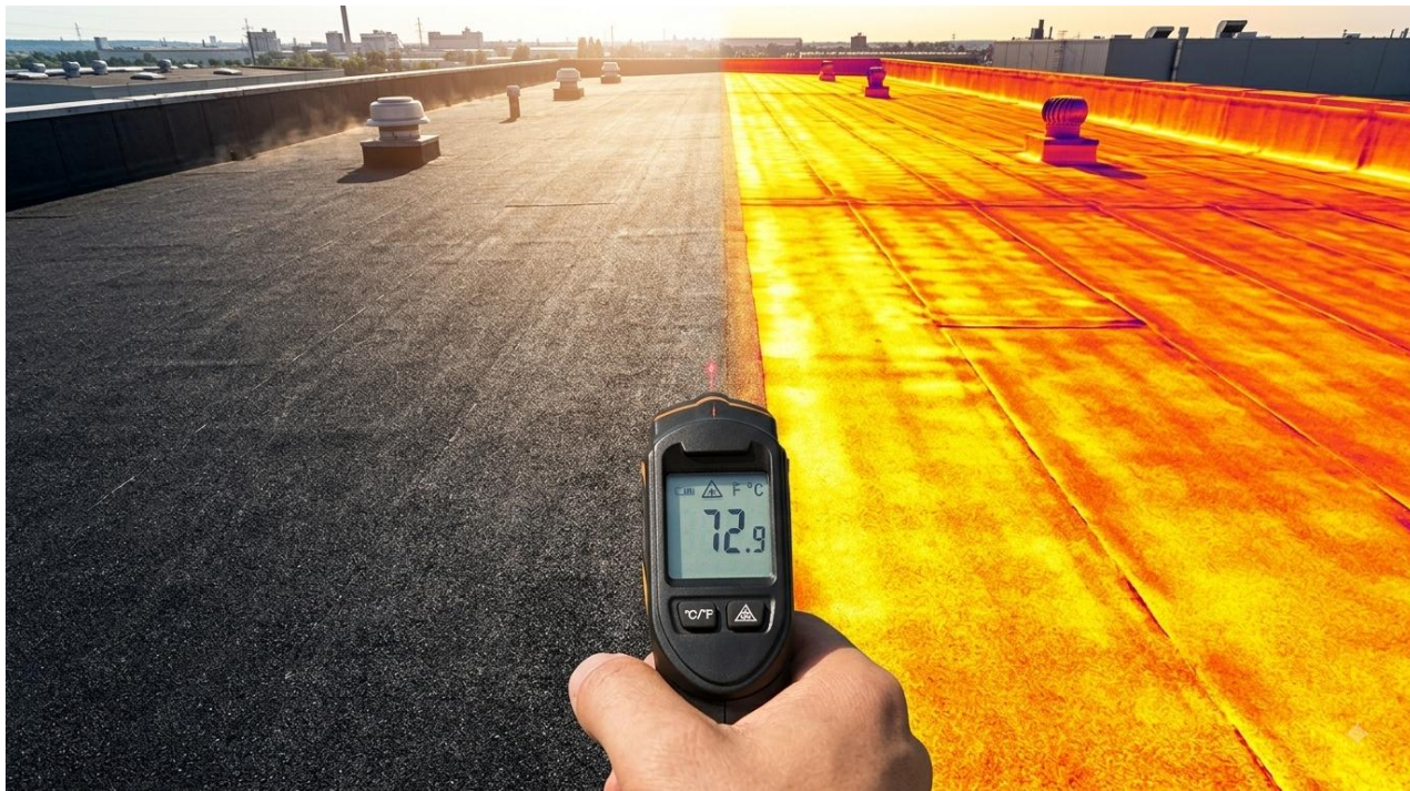
On a summer's day, a dark bituminous membrane reaches 70 to 85 °C at the surface. A thermal image instantly reveals this accumulated heat, invisible to the naked eye. (AI-generated image)
